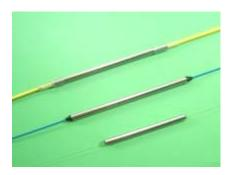
Fixed in line optical attenuator is used in optical systems where the optical power from a source is too high for the test equipment in use. it introduces an in-line fixed loss that will reduce the source power to an acceptable detection level. The attenuation level should be stable with temperature and wavelength for a stable reliable system.
