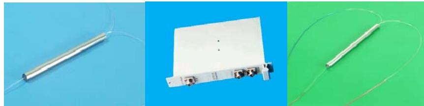
Fused WDM Filter Module (Fused Biconical Taper Process) combines light sources and emits at different wavelength into an optical fiber. They are manufactured using Fused Biconical Taper (FBT) process. Our Fused WDM Filter Module Series are ultra reliable devices featuring high isolation, low insertion loss, and high port isolation over wide ranges of temperature and wavelength.
