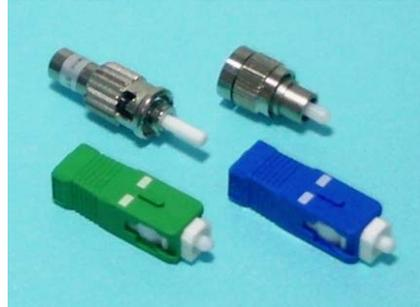
Optical Terminators are used to terminate unused **fiber connector** ports in fiber optic systems so optical terminators unwanted reflections are not introduced back into the system. It is used in fiber optic network to install on the possibly unused ports. In fiber optic network there may be unused ports in the whole system, such unused ports will create unwanted return loss and degrade the whole network performance.
