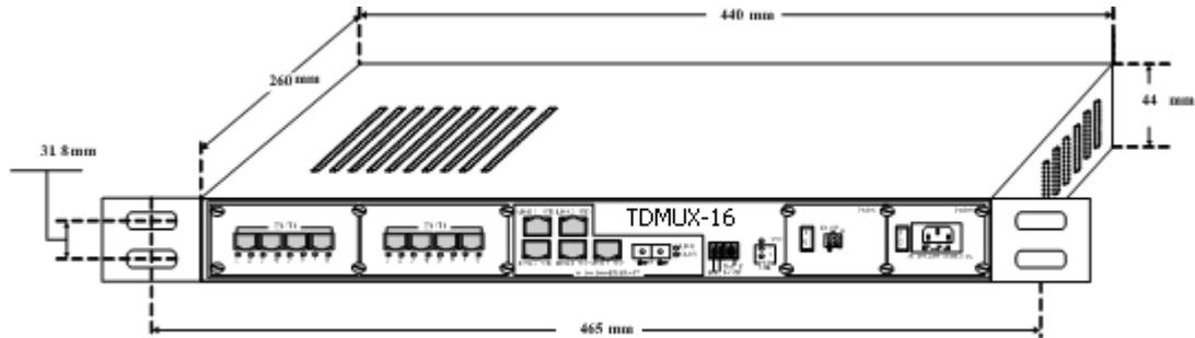
Fig.3.1-1 Mechanical dimensions
