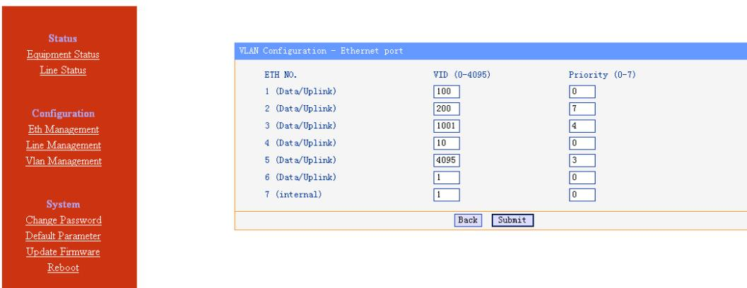
Fig 5.2-4 VLAN management interface (2)- Ethernet port configuration
