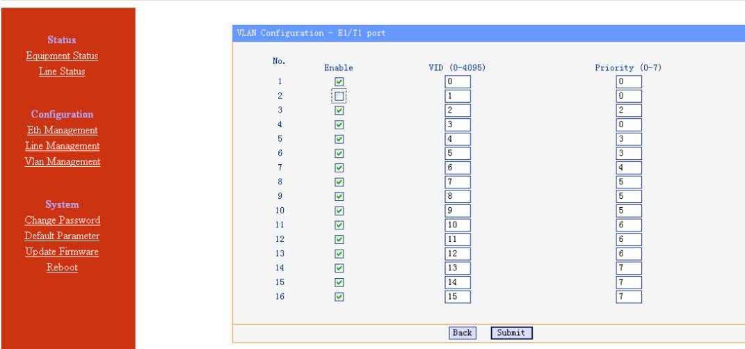
Fig 5.2-5 VLAN management interface (3)- E1/T1 port configuration
