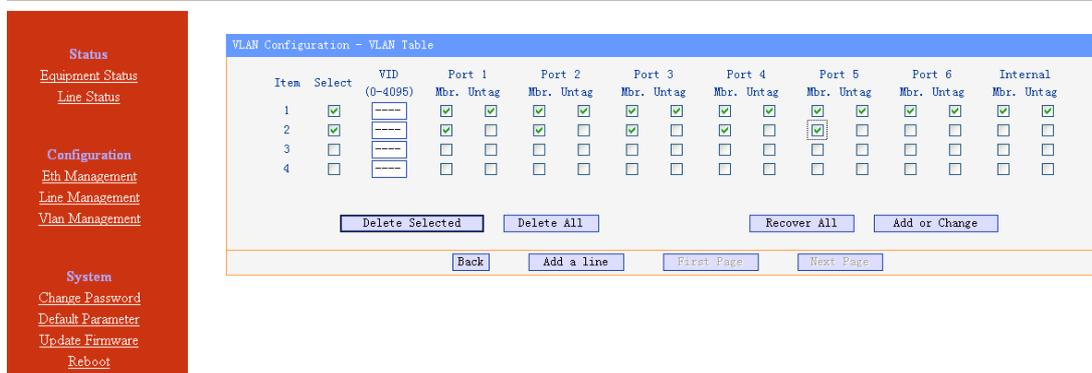
Fig 5.2-6 VLAN management interface(4)- VLAN table
