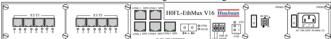
Fig. 2.4-1 Front panel of H0FL-ETHMUX V16
