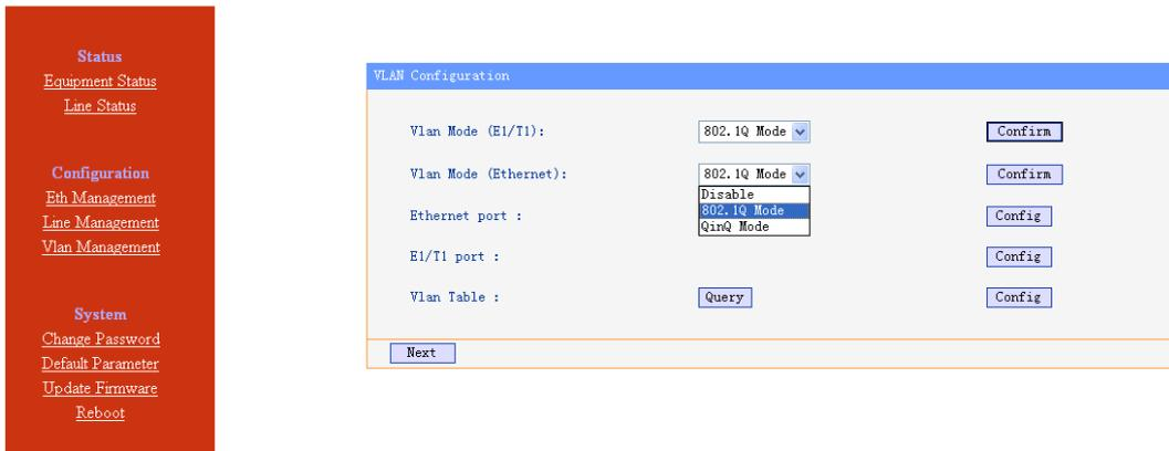
Fig 5.2-3 VLAN management interface(1) –VLAN configuration
